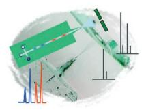
A coupling coup: A novel microfluidic chip with an integrated nanospray emitter enables the first dead-volume-free coupling of glass-chip laboratories with mass spectrometry. An electrophoretic version of the system may be suitable for the separation and analysis of drugs, for example, and has potential for the highthroughput analysis of miniscule amounts of samples.
